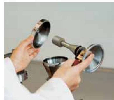
Open the vacuum tap and flame inside the funnel. Close the vacuum tap and flame the lid.
