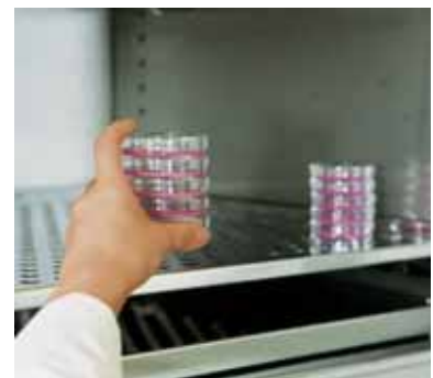
Incubate the nutrient pad in the petri dish with the lid right side up (do not invert)
