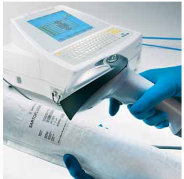
Sartocheck 4 allows easy and reliable data entry via barcode scanner (optional)
