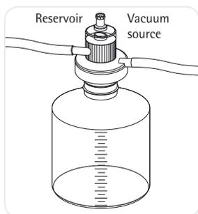
Place Sartolab® 150v on the bottle neck. A vacuum is automatically created when used with a water jet pump or other vacuum source.
