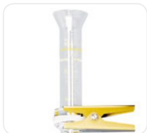
This filter holder is available in two versions differing from each other only in the type of the filter support. The filter with glass frit ensures uniform distribution of retained particles and is therefore recommended, when the residue on the filter surface is of interest. Because it is easy to clean, the device with the PTFE-coated screen support is preferable when the filtrate is required, or when liquids difficult to remove from glass frits must be
