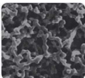
Polyamide membrane filters are hydrophilic and chemically resistant to alkaline solutions and organic solvents. They are therefore recommended for the particle removal from aqueous solutions and solvents for
