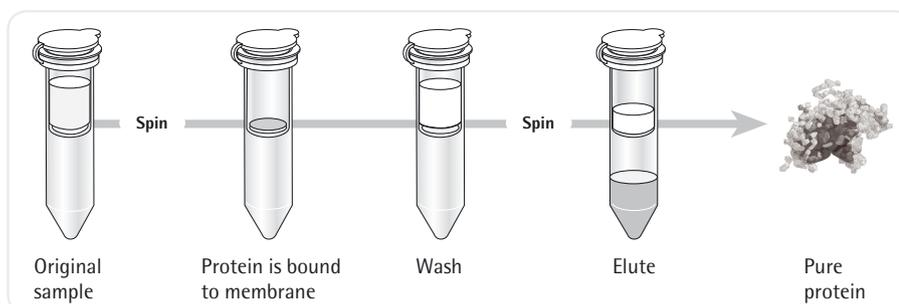
Fast and easy protein purification with Vivapure<sup>®</sup> spin columns
