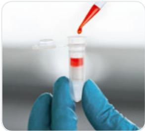
All spin columns can conveniently be used in a centrifuge. For processing larger sample volumes, e. g. from diluted cell culture supernatants, the Vivapure® maxiprep spin columns can additionally be run with a peristaltic pump collar (VS-PPCSC).
