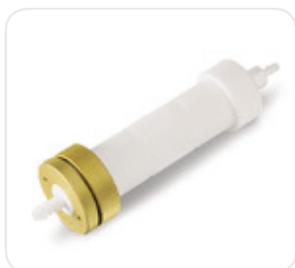
The holder hinders the release trace elements into the filtrate and is resistant to almost all chemicals. The fluoroelastomer O-ring in the top part allows easy hand tightening, and can be replaced by a PTFE
