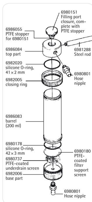
A practical filter holder for many laboratory filtrations. It can be attached to a tripod with the help of a steel rod which can be screwed in. The hose nipple is screwed into the side of the top part, leaving room for a large filling opening. This makes pouring in the sample easier, and the sample can be refilled without removing the tube connection to the pressure source. Leak-proof sealing is achieved by hand-tightening the
