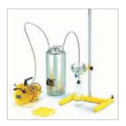
This holder is very often used in laboratories for particle removal and for sterile filtration of several liters of volume. It has a stable construction and is easy to operate. The large filtration area of 130 cm² ensures high flow rate for the total filter volume. The supplied unscrewable hose nipples can be replaced by  $G^3/g$  connectors, if systems with particularly practical handling is required.
