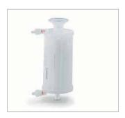
Sartobind® ion exchange capsules with 4 mm bed height are designed to remove contaminants, e. g. DNA, host cell proteins, endotoxins, leached ligands and viruses, at accelerated flow rates in flowthrough mode. This is a direct result of negligible mass transfer effects and is made possible by the > 3  $\mu m$  macroporous membrane. The design allows for robust chromatographic separations and drastically reduced validation costs.
