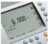
PP-15 pH Meter for pH and ORP Measurements
