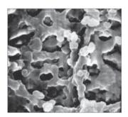
Gelatine filters in conjunction with the MD8 air samplers (gelatine filter method) are used for collecting of airborne microbes and viruses. Gelatine filter disposables are individually packed, pre-sterilized and ready-to-connect units, each consisting of a gelatine membrane filter and a holder. Gelatine membrane filters are still available as filter discs, suitable for the filter holder 17655 (80 mm diameter) supplied with the MD8 airscan® air samplers, as well as in smaller diameters.
