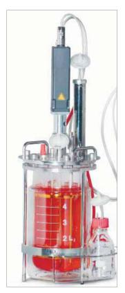
Re-usable complete filtration units with naturally hydrophobic PTFE membrane for reliable sterile venting of small fermenters and of containers for culture media.
