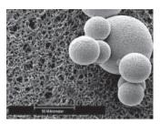
Chromatography gel beads (right) are shown on top of a membrane adsorber in this SEM picture. The membrane adsorber pores are over 50 f larger than bead pores.
