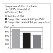
Newly developed, ready-to-use pressure filtration units offering maximum convenience for the sterile filtration of 0.1 to 50 liters of buffers, infusion solutions, tissue culture solutions, sera and other solutions containing proteins. No more problems with air bubbles in the liquid. A hydrophobic PTFE membrane validated for sterile air filtration allows for effective air bubble collection at the highest point upstream.
