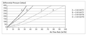
Air flow rates at atmosperic pressure Sartofluor® mini 0.2  $\mu$ m, Type 5181507T7, T8, T9, 5181407T7
